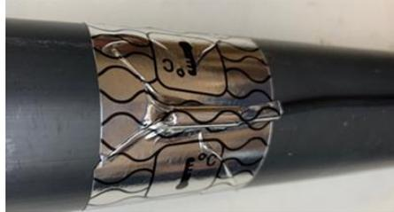
Fig 4 – Temperature Probe Installation
