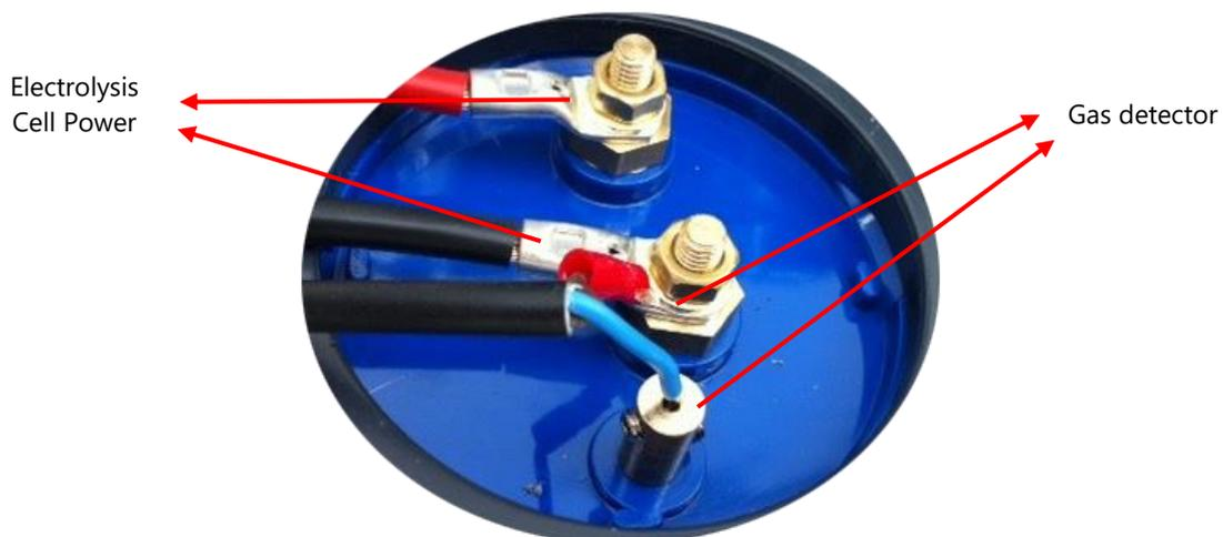
Fig 5 – Electrolysis Cell Connection Terminals
